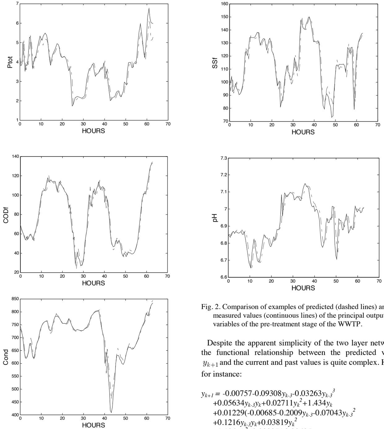
Fig. 2. Comparison of examples of predicted (dashed lines) and measured values (continuous lines) of the principal output variables of the pre-treatment stage of the WWTP.
